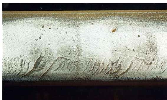
Figuur 3-6: Head check (ProRail, 2016)
