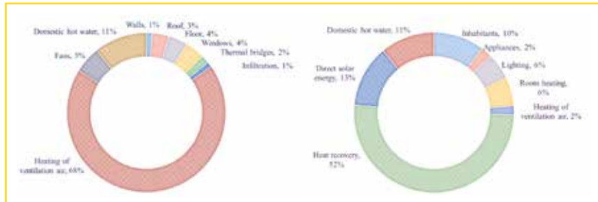
Figure 3: Distribution of energy losses and gained energy in the room
